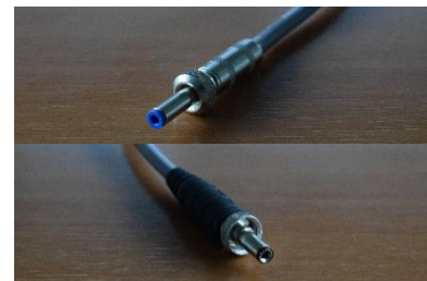
Figure 8: The two connectors on the PDM cable. Blue connector at the charging cradle side, black connector at the PDM side
