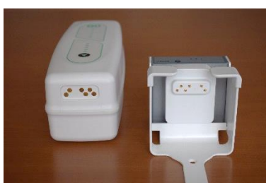
Figure 3: The contacts between the battery and the charging cradle
