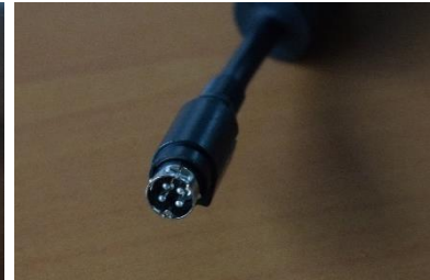
Figure 6: The four-pin connector with the locking mechanism
